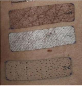
Figure 10. This image shows a close up photograph of representative tapes illustrating skin oil (sebum) striking through the tape. However this did not appear to affect the performance of the samples. Shown are Tapes 1, 2, and 3.
